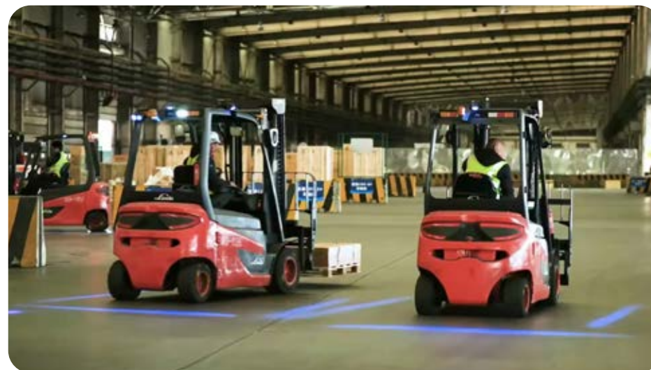
"Installation of warning light strips on forklifts": By projecting light beams onto the ground, a clear boundary is formed around the forklift, facilitating the alerting of surrounding personnel, the forklift itself, and other forklifts to promptly avoid collisions.
