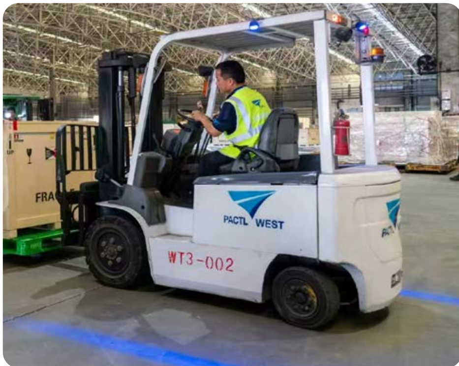
"Installation of warning light strips on forklifts": By projecting light beams onto the ground, a clear boundary is formed around the forklift, facilitating the alerting of surrounding personnel, the forklift itself, and other forklifts to promptly avoid collisions.
